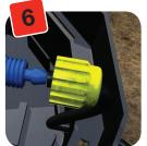
The AQUAvalve can now be connected to the 6mm pipe. Unscrew the yellow collar and push the pipe through it. Push the 6mm pipe on to the nozzle of the AQUAvalve and then replace the vellow collar by screwing it onto the AQUAvalve.
