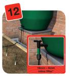
Image 12 shows the AQUAbox Spyder connected to a 200 litre water butt using a 16mm-6mm In-line filter supplied with your kit. Take a length of 16mm pipe or standard hosepipe 100mm/4 inches in length...\*\*note this pipe is not supplied with your kit\*\*...Push the hosepipe on to your tap, then connect the filter to the pipe and then take your 2 meters of 6mm pipe connected to your AQUAbox Spyder and connect it to the other end of your filter.
